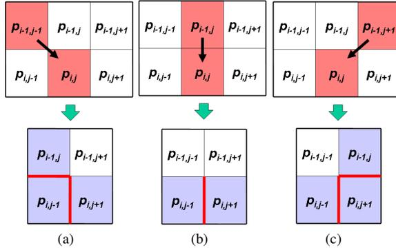
**Figure 9:** Calculating the three possible vertical seam step costs for pixel  $p_{i,j}$  using forward energy. After removing the seam, new neighbors (in gray) and new pixel edges (in red) are created. In each case the cost is defined by the forward difference in the newly created pixel edges. Note that the new edges created in row  $i-1$  were accounted for in the cost of the previous row pixel.
