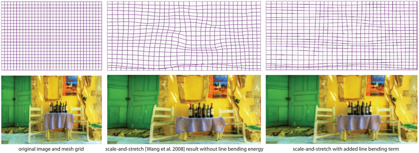
**Figure 16:** Demonstration of the effect of the line bending energy term in the scale-and-stretch warping technique of [Wang et al. 2008]. Note how adding the energy term prevents strong grid line bending and produces a less distorted retargeting result.
