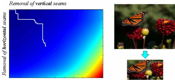
**Figure 12:** Optimal order retargeting: On the left is the transport map  $\mathbf{T}$  of the retargeted image on the right. Given a target size, we follow the optimal path from the target size to  $(0, 0)$  (on the upper left corner) and apply either a vertical or a horizontal seam removal to obtain the retargeted image (see example of white path on  $\mathbf{T}$ ).
