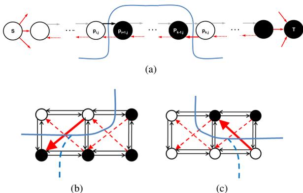
**Figure 14:** Using infinity edges (red) in the graph construction maintains the seam constraints. Horizontal infinity arcs maintain monotonicity (a) - see details in text. Diagonal infinity arcs maintain connectivity. If the cut skips more than one pixel to the left (b) or right (c) - a diagonal infinity arc from a source node (white) to a target node (black) must be cut.
