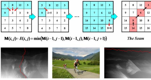
**Figure 8:** Top: example of creating the vertical accumulated energy map  $M$  and backtracking to find the seam. Bottom: visual representation of the vertical and horizontal maps of an image (middle) and the optimal seams found.
