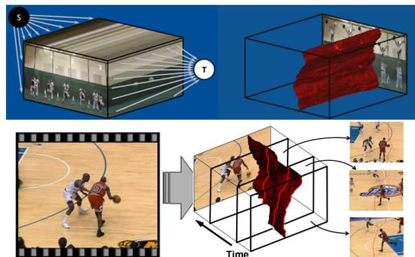
**Figure 15:** Top: the construction of a graph on a video cube guarantees the graph-cut will find a connected and monotonic manifold in the volume. Bottom: The intersection of the manifold with each video frame defines the seams on the frame.
