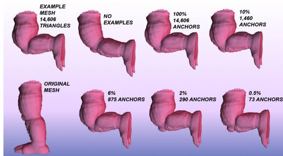
**Figure 7:** The effect of using different amount of anchors when deforming the original mesh using one example. Using just 2% of the triangles as anchors produces a muscle bulging effect almost indistinguishable from that produced with 100% anchors.
